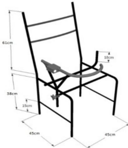
**Fig. 5.1: Base Frame with Tab support (all dimension in cm)**
