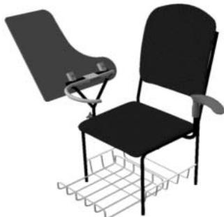
**Fig. 5.2: Isometric view of the Designed Tabloid Chair.**
